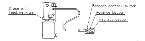
③ In case oil could not be delivered to develop pressure, place the pump horizontally (normal position) and push the rubber bag through the hole (8mm dia.) on the tank cover end with a rod having a round end, with attention that the rubber bag does not get hurt, and at the same time do inching operation with the pendant switch.
