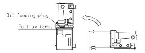
$\odot$  How air may accumulate in the pump (rubber tank) when hydraulic equipment are connected together with? Always check and confirm before use that the oil tank is full.
