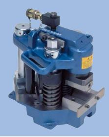
FM-30 is a forming machine with outstanding workability, unnecessary for die replacement. It is a compact, high-performance machine that can cut and bend stainless steel angle material of 75 mm (width) x 6 mm (thickness).
