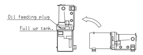
⊚ How air may accumulate in the pump (rubber tank) when hydraulic equipment are connected together with? Always check and confirm before use that the oil tank is full.
