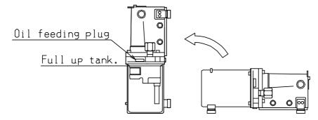
② In case even if the tank is full oil cannot be delivered to develop pressure, stand the pump with the tank end down and do inching operation (intermittent switching) with the pendant switch about 10 to 11 times.
