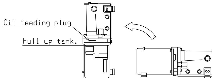
©How air may accumulate in the pump (rubber tank) when hydraulic equipment are connected together with? Always check and confirm before use that the oil tank is full.
