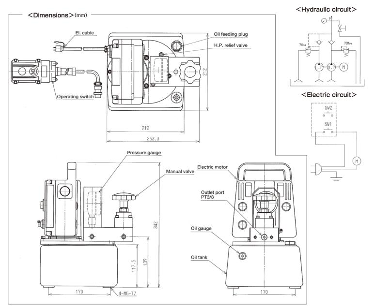
UP-45SVG-4 (Pressure gauge, Standard tank 3ℓ) UP-45SVG-4L (Pressure gauge, L tank 5ℓ) UP-45SVS-4 (Pressure gauge, Pressure Switch, Standard tank 3ℓ)
